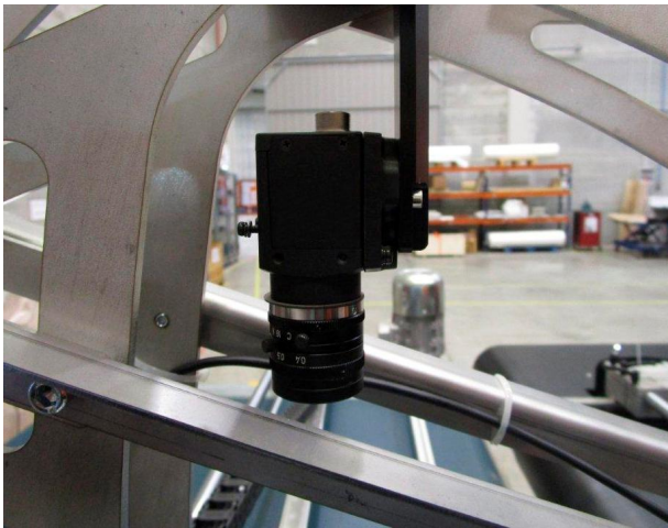
The Cretavision 2.0 compact camera in place
