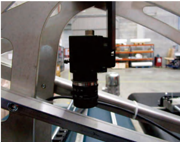
The Cretavision 2.0 compact camera in place
